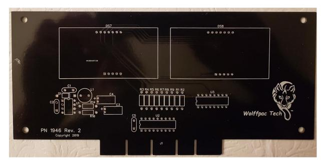
Insert U1 (MAX5033) into the board from the top side (the side with the lettering) so that one pin goes through each hole at the location labeled 'U1'. Each chip is marked with a 'U'-shaped notch on one of the short ends:
